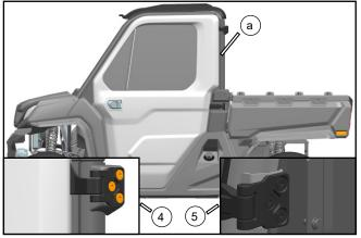
Use the stepping bolt M6×17 (14) to mount the limiting cable assy (3) on the LH/RH front door assy (2).
