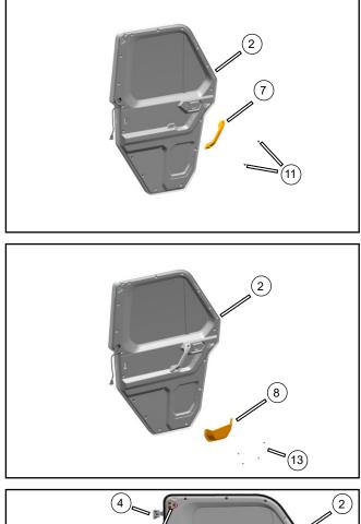
Use the inner hexagon bolt M6×20 (11) to mount the LH/RH door inside armrest (7) on the LH/RH front door assy (2).
