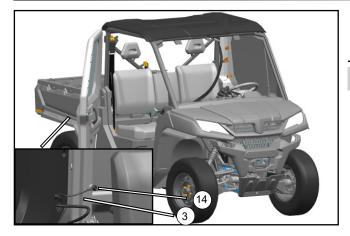
Øpen the gate, use the stepping screw M6×17 (14) to mount the limiting cable assy (3) on the frame, and connect the reserve cable plug of the electric lift door and reserve cable plug of the vehicle body.
