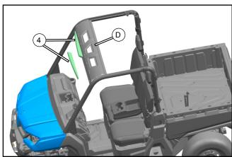
Install the windshield supporter seat (4) to the top roof mounting plate (D).
