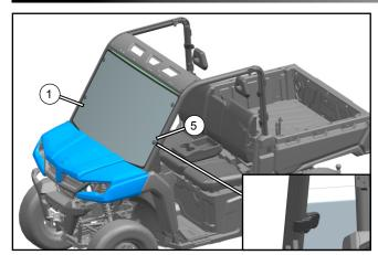
Position the front windshield assembly (1) on the top bar front assembly as shown to determine the clamp positions, then assemble each side with clamps (5). Tighten the screws sufficiently, using care not to overtighten.
