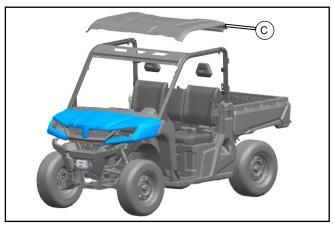
// Remove the top roof (C).
