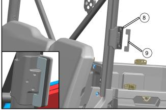
Fasten the screw cap (9) to the clamp (8).
