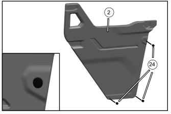
// Install three rubber mats (24) into the corresponding holes of the LH half door (2) at the locations shown.
