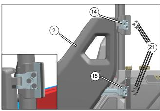
Install the left upper connecting plate assy (14) and the left lower connecting plate assy (15) on the left half door (2) to the corresponding holes of the frame.
