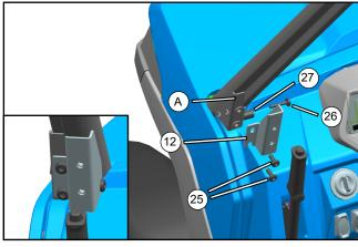
// Install the left buckle bracket assy (12) and shaft sleeve (27) on the frame cab (A) by M6x35 bolts (26), then install 2 M8x25 screws (25) onto the frame cab (A).
