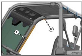
Paste the wire duct (4) and the cable tape (12) on the assembly position of the passenger side beam.
