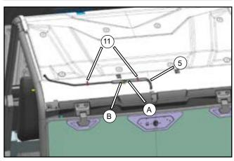
Plug the terminal (A) of the wiper motor assembly into the terminal (B) of the main cable assembly. Pass the hose (5) through the reserved hole in the front of the felt. Secure them with the tie band (11) after neat wiring.
