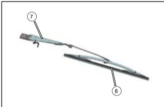
// Assemble the wiper arm (7) and the wiper blade (8).
