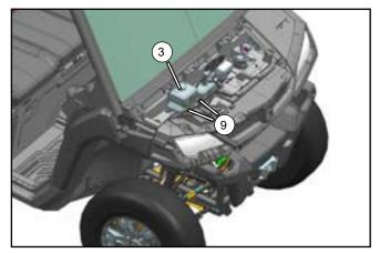
Place the water bottle assembly (3) on the assembly position and secure it with bolts M6×16 (9).
