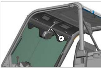
// Pass the wiper motor assembly harness (A) through the reserved hole in the front of the felt.
