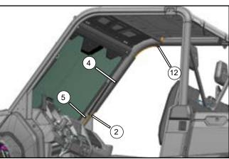
The main cable assembly (2) and the hose (5) are routed along the passenger side beam. Pass them through the wire duct (4) and fix them with the cable tape (12). Then pass them through the reserved hole on the right side of the felt.
