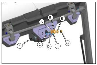
Place the wiper motor assembly (6) into the assembly position of the front windshield. Install the gasket (A), gasket (B), gasket (C), and gasket (D) in order with the bolts (E), (F) tightened. Then install the stopper nut (G).
