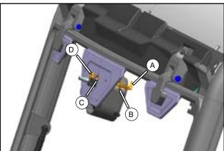
Place the adapter nozzle (A) and the gasket (B) into the assembly position of the front windshield. Install the gasket (C) and tighten it with the nut (D).
